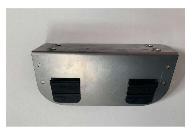
6. Fit the windage tray – this is essential to ensure any oil wash is minimised under heavy braking. The folded tags each end ensure an interference fit to stabilise the tray – fix with the 4 x M6 set screws and bend the lock tabs up as necessary to ensure they do not come loose. Putting a slight edge lift each end of the tags before fitting if you wish, will make life easier.
